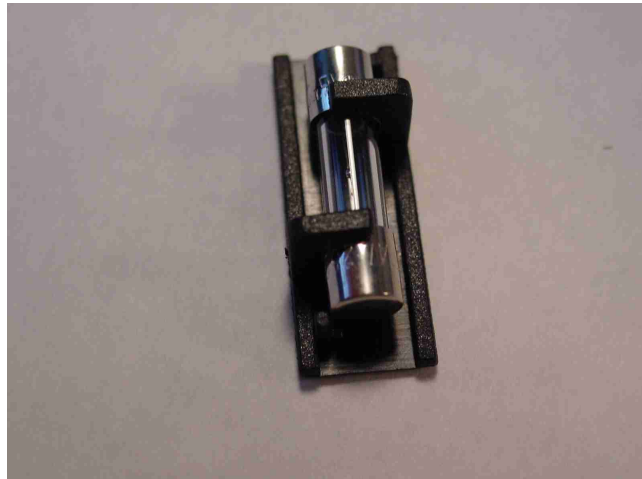
Lid of the fuse holder with inserted fuse
