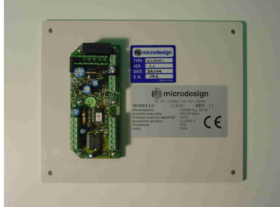
n. 1 Electronic control card, mounted on Panel
