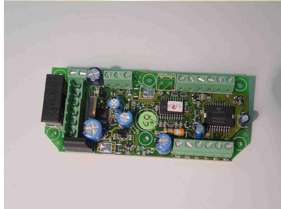
n. 1 Electronic control card, to mount on the power-supply unit (on three turrets)
