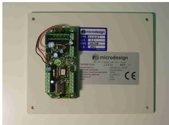
n.1 Electronic control card, mounted on the Panel with a Plug for battery charger
